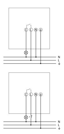
The device can be manually activated with a circuit breaker. After releasing the button (return of power) the device switches on (for at least 40 secs or for the time set on the device).
