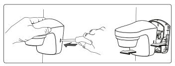
➤ Using the screwdriver, carefully loosen the snap-in hook at the side and pull the device forward.
